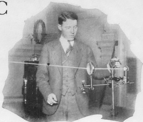
The receiving end of the photo-electric organ. Interrupted light rays from the rotating disc at the left enter the photo-electric cell and are converted into musical tones
