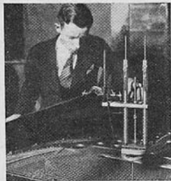
C. A. Johnson , of the E. E. Free Laboratories, with a special electro-magnetic pickup used to take the tone from a single square inch of a piano sounding board
